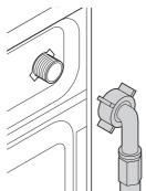
In order to prevent water leakage that may occur at the connection points, there are rubber seals (4 seals for the models with double water inlet and 2 seals for other models) attached to the hoses. These seals should be used at the tap and machine connection ends of the hoses. The plain end of the hose fitted with a filter must be attached to the tap and the elbowed end
